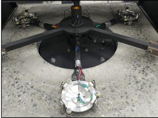
*Figure 4: Temperature test setup measuring 'in-pod' (bottom of the fabric)*
