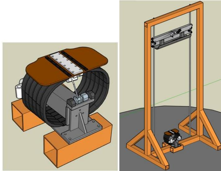
*Figure 6: Sketch of the dummy base and the free fall impact machine for airbag jackets*
