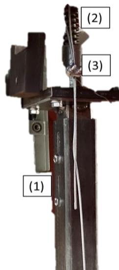
*Figure 3: System developed in addition to AART Impact abrasion machine (EN17092-1) aiming to intensify the factor impact*
