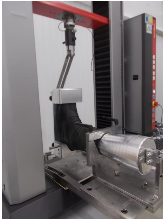
Figure 7. Bending on ankle machine for boots, flexion-extension mode.
