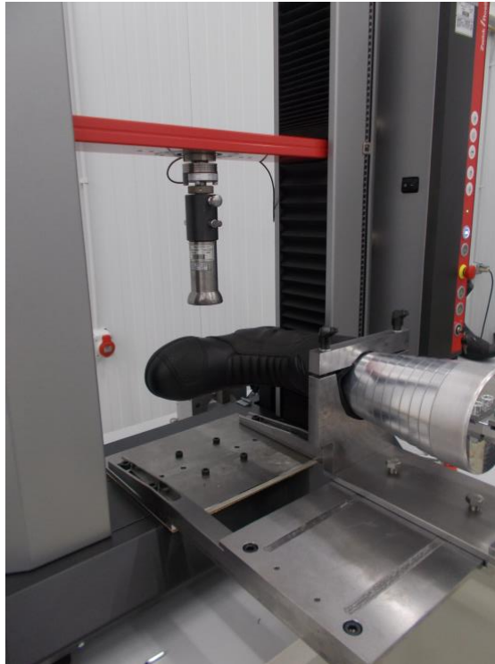
Figure 8. Bending on ankle machine for boots, eversion mode.
